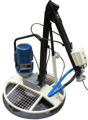
The **Concrete Power Trowel** with electric motor is a high efficiency, light weight machine for floating & troweling concrete surface. the machine can be operated at two speeds 115 and 57 R.P.M. to obtain the desired output. This machine is provided with two types of finishing tools. A disc for floating and a set of four blades for troweling. to obtain fine finish the blade angle should be control.
