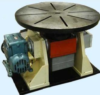
**Nextgen Welding** turntables, or welding rotating tables, provide a high-precision, low-cost method of rotating a pipe, vessel or industrial work piece around a vertical axis. Rotary turntables are used for precise positioning in the flat or horizontal position. Floor turntables are well suited for welding, flame cutting, X-ray and machining application.
