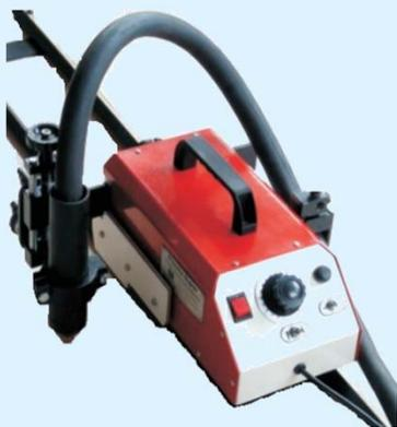
Nextgen straight-line track cutting system is available in plasma or oxyfuel configurations. It cuts up to 100mm thick plate with an oxyfuel torch and up to 25 mm thick plate with a plasma power source up to 100 amps.
