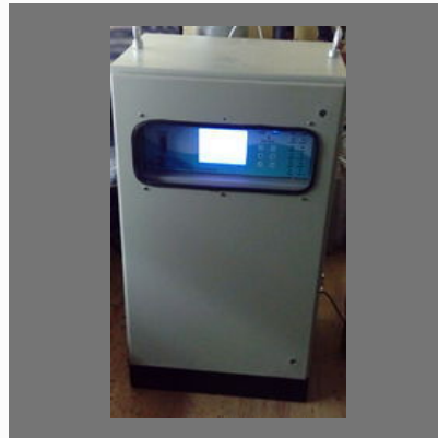
Online Continuous Emission Monitoring System OCEMS
