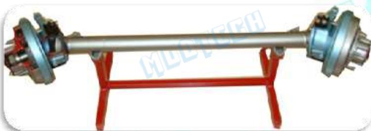
*This model is made out of original used light vehicle, suitably sectioned to show the action of Differential gear box and Brake drums in Rear axle. A Crank handle is provided to demonstrate the model. The whole model is mounted on a sturdy iron frame.*
