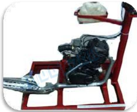
The petrol engine setup will be prepared by using good working condition engine with all the fittings of the engine along with silencer, air filter, fuel tank ,electrical wiring with ignition switch etc., all mounted on to a sturdy iron frame with caster wheels (mobile trolley) .
