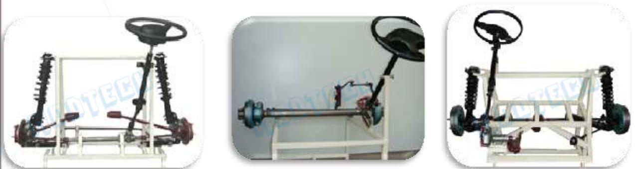
*This model is made out of full size original parts, suitably sectioned and to demonstrate the working of Steering wheel worms, Steering arm, etc., The Arrangement Of Wheels And Axle Connecting To steering system will be done so the movement of the wheels when rotating the steering wheels can be displayed .*
