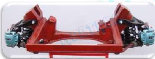
*This model is made out of original used parts, will be suitably sectioned And Arranged to demonstrate the internal construction details showing the minute information With Suspension Strut with spring and shock absorber, disc brake, callipers drive shaft etc., and working of the same can be shown, the model will be suitably painted and The entire model is mounted on a sturdy iron frame.*
