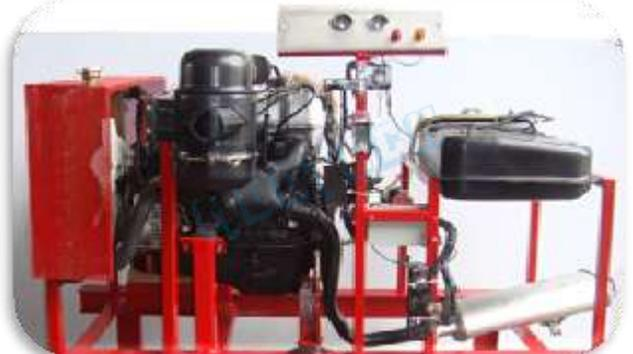
The Four stroke petrol engine setup will be prepared by using good working condition multi cylinder car engine with all the fittings of the engine along with radiator, silencer, air filter, starter, battery, alternator, indication meters, fuel tank ,electrical wiring with ignition switch etc., all mounted on to a sturdy iron frame with caster wheels (mobile trolley) .
