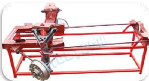
*This model is made out of original used parts, will be suitably sectioned And Arranged to demonstrate the internal construction details showing the minute information With Suspension System with longitudinal torsion bar arrangement, shock absorber, etc., and working of the same can be shown, the model will be suitably painted and The entire model is mounted on a sturdy iron frame.*
