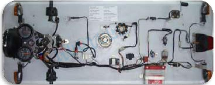
*giving connection the working of individual parts such as Self, Horn, Head lights, Tail lamps, Parking lamps, Side indicators, Brake light, Distributor, Sparks of spark plugs, etc., can be demonstrated. The parts sectioned to show the internal constructional details. This is a working demonstration model.*
