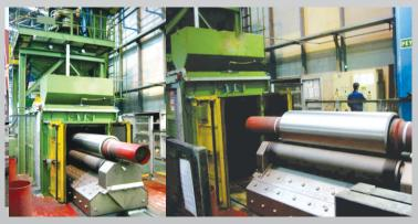
This machine is suitable for blast cleaning of rolls upto 800 mm width with multiple centrifugal blast wheels strategically positioned to fire shots at high velocity on to the moving roll with facility of variable job conveying speeds. The various grades of etching are repeatedly obtained to maintain the rolled surface quality
