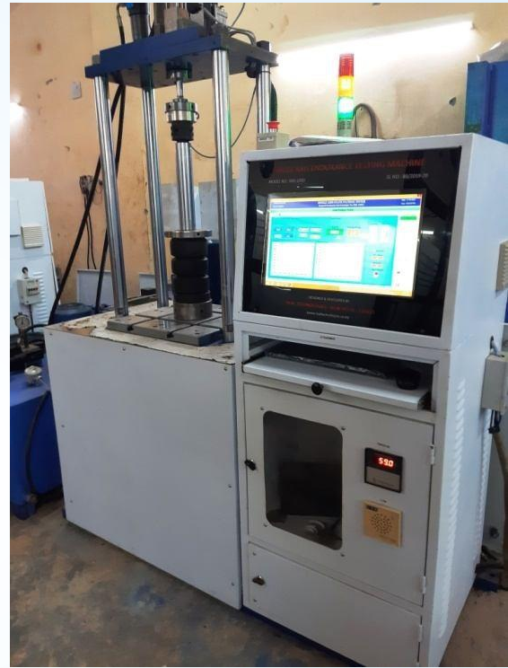
RBS -10000 (100 kN) without heating chamber
