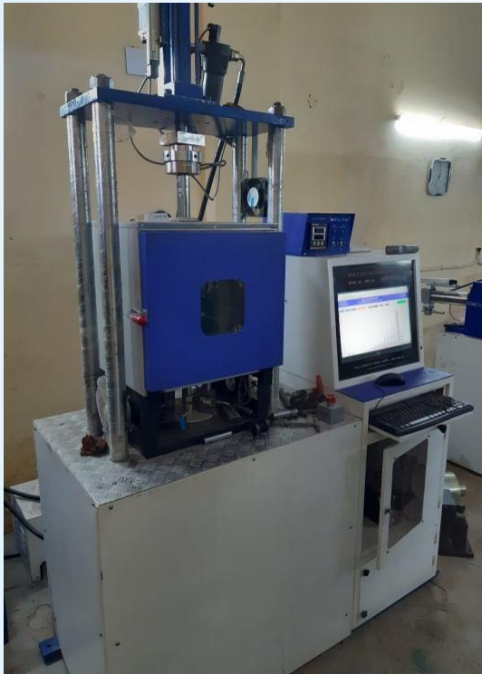
RBS -1000 (10 kN) with heating chamber
