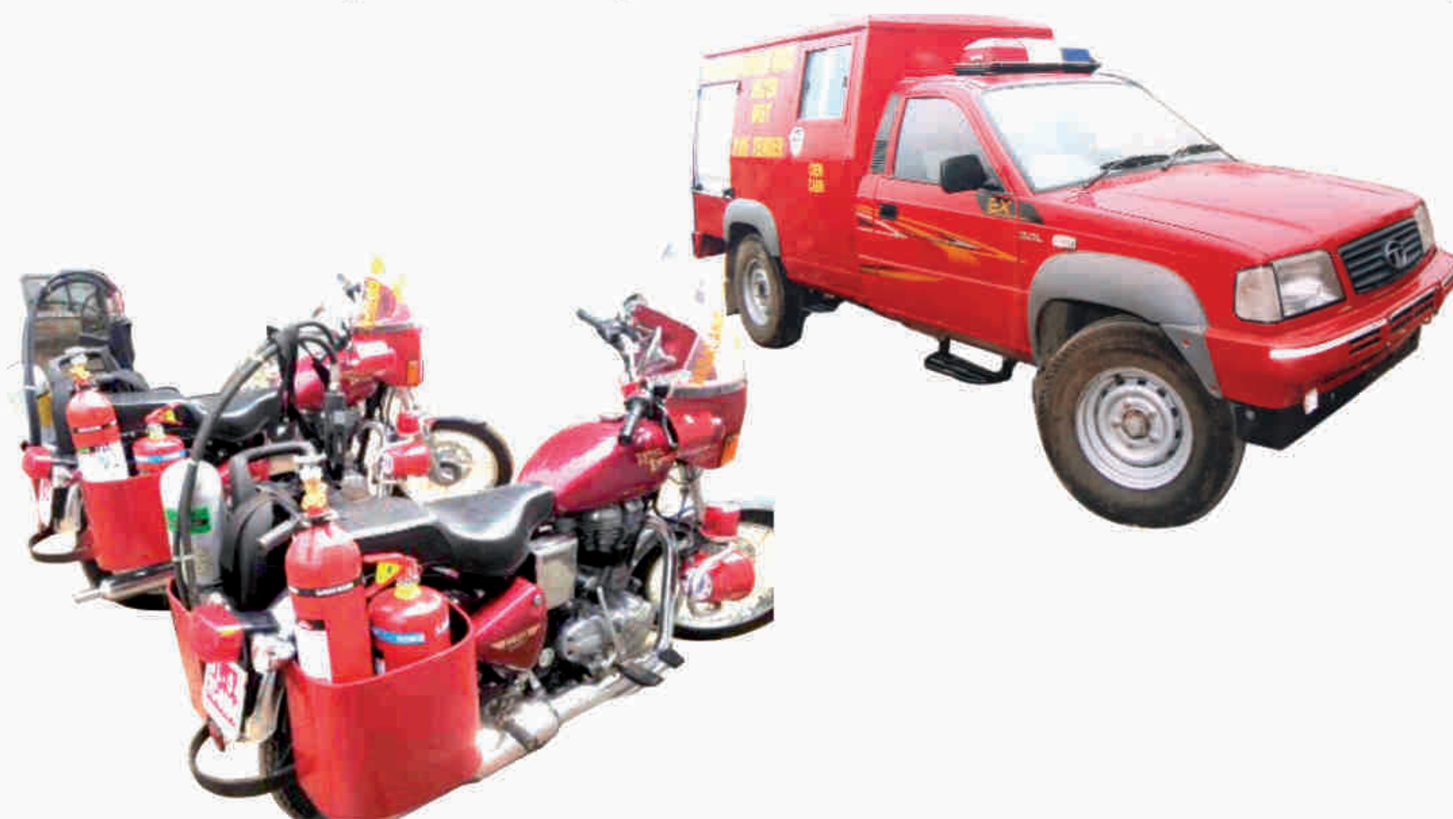
Rescue Bike/Vehicle (with Back Pack Water Mist)
