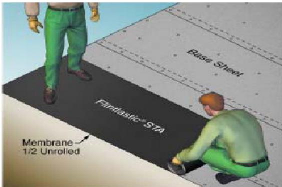
4. Membrane application by unrolling the roll and aligning the side laps. Reroll the roll halfway, standing on the unrolled prevent shifting.
