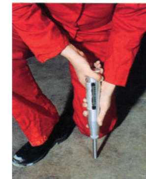
Schmidt hammer test
