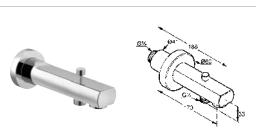
KLUDI bath filler with diverter DN 20 wall fastening flow class B aerator M 28 x 1 autom. diverter shower/bathtub protected against back flow with push-on rosette projection 170 mm
