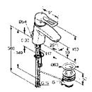
KLUDI MX single lever basin mixer DN 10 open ring lever single hole mounted flow class A s-pointer aerator M 24 x 1 ceramic cartridge with hot water limitation pop-up waste G 1 1/4 flexible hoses G 3/8
