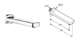
KLUDI Q-BEO bath filler DN 20 wall fastening projection 220 mm s-pointer aerator M 24 x 1 flow class D separate connector G 3/4 for pre-assembly G 3/4
