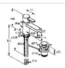
KLUDI ZENTA XL single lever basin mixer DN 10 solid lever single hole mounted flow class Z s-pointer eco-aerator M 24 x 1 ceramic cartridge with hot water limitation pop-up waste 6 1 1/4 rapid installation set flexible hoses G 3/8 P-IX 18634/IA
