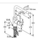
KLUDI L-INE single lever sink mixer DN 10 solid lever, single hole mounted flow class Z caché Laminar-flow-regulator M 24 x 1 ceramic cartridge with hot water limitation swivelling spout (220°) pull-out telescopic hand spray with horizontal guidance (245 – 315 mm) protected against back flow shank fastening flexible hoses G 3/8 noise level I
