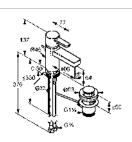
KLUDI ZENTA single lever basin mixer DN 10 solid lever single hole mounted flow rate 4,8 l/min PCA-aerator M 24 x 1 ceramic cartridge with hot water limitation pop-up waste G 1 1/4 rapid installation set flexible hoses G 3/8 P-IX 18634/IA WELL Reg. Nr. WA1003420101104
