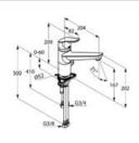
KLUDI OBJEKTA multi single lever sink mixer DN 15 for use with displacement heaters solid lever single hole mounted ceramic cartridge with hot water limitation flow regulator M 24 x 1 flow rate 5 l/min swivelling spout (360°) one connection for washing machine or dishwasher
