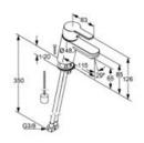
KLUDI LOGO NEO single lever basin mixer DN 10 solid lever single hole mounted flow class Z eco-aerator M 24 x 1 ceramic cartridge with hot water limitation retractable chain rapid installation set flexible hoses G 3/8 noise level I P-IX 19334/IZ
