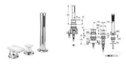
KLUDI E2 single lever bath- and shower mixer DN 15 solid lever stand assembly three hole tiles deck mounted installation flow class DB s-pointer aerator M 24 x 1 ceramic cartridge with hot water limitation autom. diverter shower/bathtub retractable hand shower high pressure supply hose G 1/2 x G 1/2 x 600 mm protected against back flow for bathtub rim mounting unit 7580200-00 or mounting plate 7614946-00
