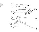
JOOP! head shower DN 15 wall fastening flow class B quick and easy cleaning system shower spray connection G 1/2
