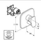
KLUDI AMBA concealed single lever bath and shower mixer concealed valve with functional unit solid lever wall fastening autom. diverter shower/bathtub ceramic cartridge with hot water limitation flow class DC noise level I PA-IX 18967/IDC
