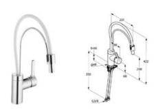
KLUDI BINGO STAR single lever sink mixer DN 15 solid lever single hole mounted flow class Z PCA Caché-Laminar-flow regulator M 16,5 x 1 ceramic cartridge with hot water limitation swivel (360°) — removable spout protected against back flow rapid installation set flexible hoses G 3/8 noise level I
