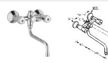
KLUDI SPECIAL bath-and shower mixer DN 15 handle Terralux ABS (15) wall fastening flow class BA swivelling spout 200 mm aerator M 22 x 1 autom. diverter shower/bathtub protected against back flow shower outlet G 3/4 chrome
