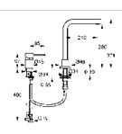
KLUDI L-INE single lever sink mixer DN 10 solid lever, two hole mounted flow class Z PCA Caché-Laminar-flow regulator M 16,5 x 1 ceramic cartridge with hot water limitation swivelling spout (360°) flexible hoses G 3/8 rapid installation set noise level I
