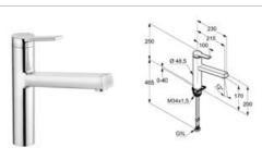
KLUDI ZENTA single lever sink mixer DN 15 solid lever single hole mounted flow class A s-pointer aerator M 24 x 1 ceramic cartridge with hot water limitation swivelling spout (360°) with shank fastening flexible hoses G 3/8
