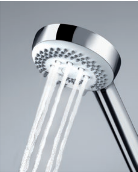
Smooth The smooth spray is generated by six mini-aerators, which mix air into the water, thus ensuring a gentle stream of water.
