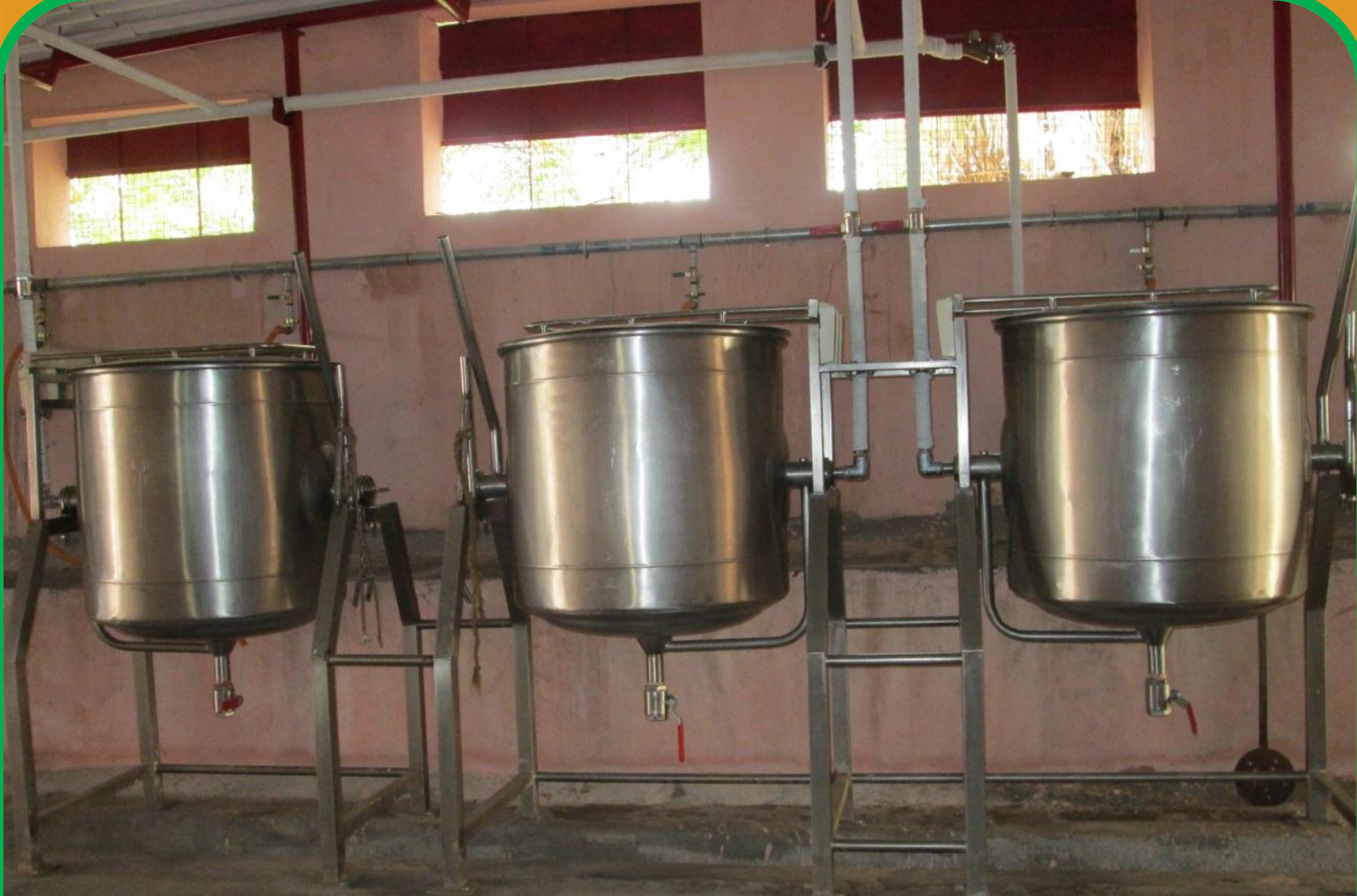
SS 100.KG Raw Rice cap Steam Cooking Vessel
