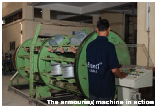
The armouring machine in action
