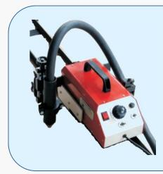
**Nextgen** straight-line track cutting system is available in <u>plasma</u> or oxyfuel configurations. It cuts up to 100mm thick plate with an oxyfuel torch and up to 25 mm thick plate with a plasma <u>power source</u> up to 100 amps. The small, <u>portable unit</u> is suitable for use on job sites and eliminates the hand cutting of long straights. The track can be extended in 1500mm sections to the required length. Adjustable torch heads can cut bevels and V's from 0 to 45 degrees.
