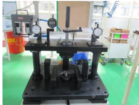
Checking gauge systems Value engineering SPP
