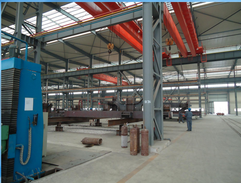
行车/Crane 起吊重量 Lifting amount: 30t
