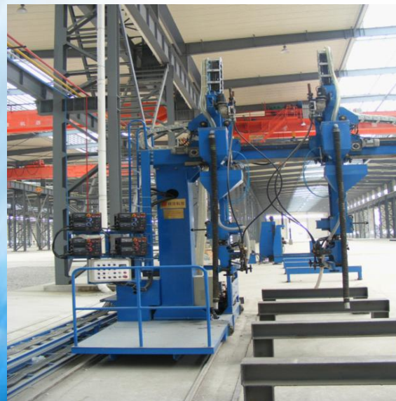
悬臂式双弧双丝埋弧焊机 Hanging SAW machine with double arch and wire Working distance: 18m
