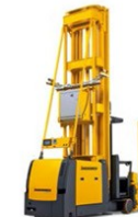
Automatic very narrow aisle truck EKXa max. lift height: 14,000 mm max. capacity: 1,500 kg
