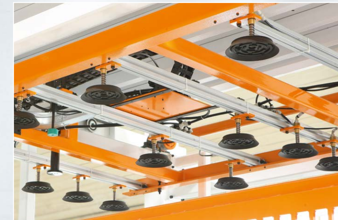
Suction cup device for lifting raw metal sheet: Is an arm with the grip placed over the loading pallet. The duty of this arm is to lift the raw metal sheet to permit the entrance of the comb device under the metal sheet lifter and deposit it on this comb device.
