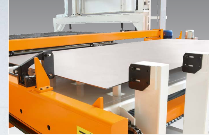
X Reference Arm: This arm provide you to reference metal sheet and precise handling for the suction cups.
