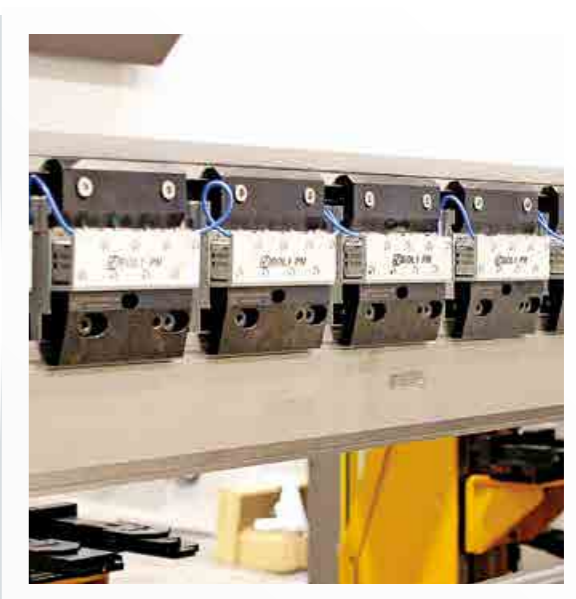
Pneumatic Tool Clamping System (O) Pneumatic tool clamping systems press and center the tools automatically with the help of the pressurized air. These are perfect solutions to shorten the setup timing and for automated press brakes.
