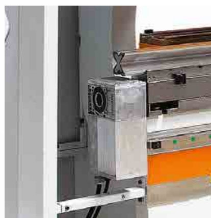
CNC Motorized Crowning System (*) CNC crowning system that communicates with the CNC controller, performs crowning automatically and enables the part to be at even bending angle at any given point. * Up to 400 TN optional. From 400 TN and above standard.
