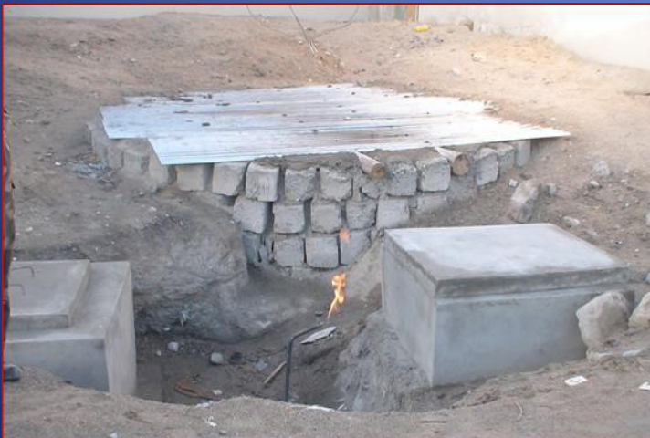
Spot test for inflammability of biogas
