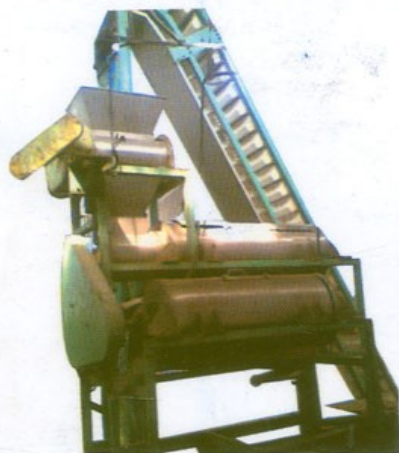
DOUBLE STAGE PULPER WITH ELEVATOR
