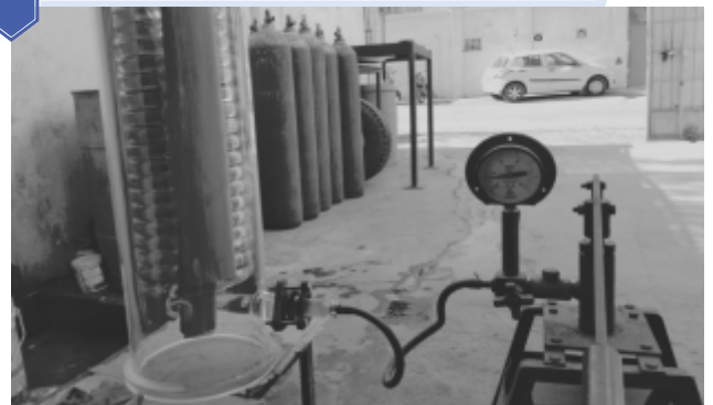
08 Condenser Hydro Pressure Testing
