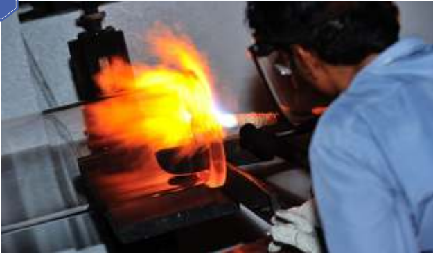
01 Glass Big Flange Making Process
