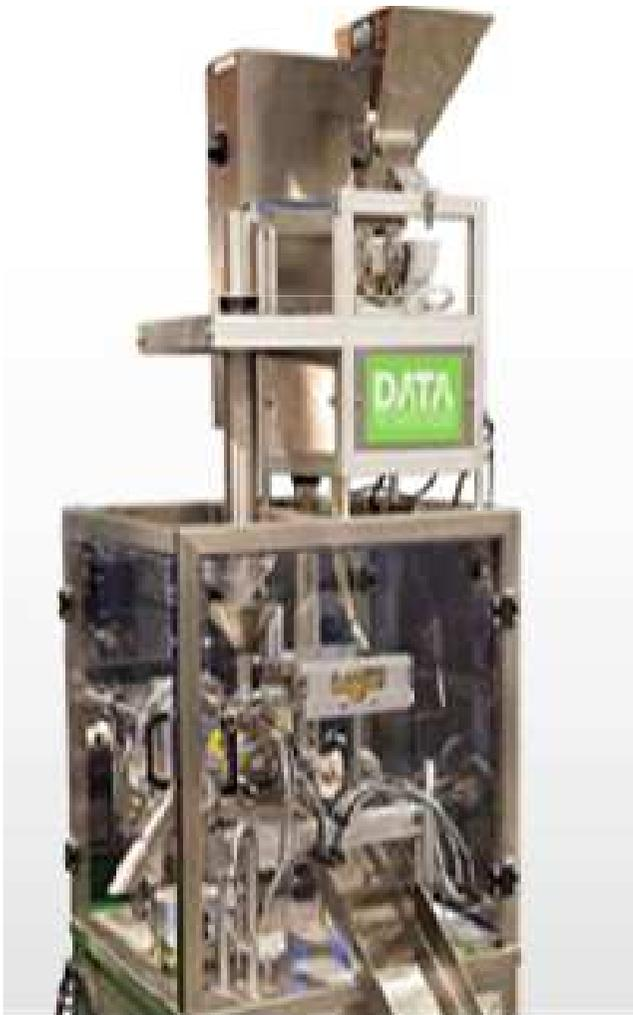
✓ Precisely counts all seed shapes from 1 mm and up to 25 mm
