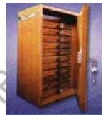
Temperature is controlled by a thermostat and it and be read on dial type thermometer. Temperature range:  $50^{\circ}$  C to  $250^{\circ}$  C to  $5^{\circ}$  C and equipment is workable on 220 VAC 50 Hz phase or 440 volts A supply.
