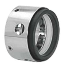
These Seals can be easily assemble or dismantled through circlip provided & cab be change to Balance version of its type merely by changing the carbon face only & an be provided with single, double or tandem arrangement worth external seal support systems & devices.
