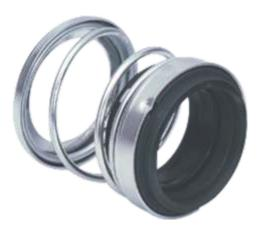
The seal can be use regardless of direction of rotation since the driving torque is not transmitted through the coil spring. The required driving torque is enhanced through the unique rubber bellow which fits on the shaft through the interference fit between the collar, rubber bellow & the shaft.
