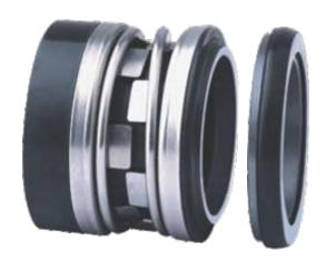
The seal can be use regardless of direction of rotation since the driving torque is not transmitted through the coil spring, The required driving torque is enhanced through the unique rubber bellow which fits on the shaft. There are no bonded Joints and all the face materials are interchangeable without having to modify any dimensions.
