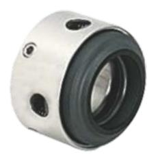
springs do not come in contact with the circulating media & therefore can be use for corrosive or abrasive media sealing. The compact design eliminates the requirement of extra radial & axial space for its installation.
