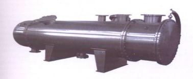
When gas is having design pressure more than 50 bar, then it is recommended to design the Heat Exchanger with Gas on Tube Side & water on shell side. It is a removable tube bundle, outside packed floating tube sheet design
