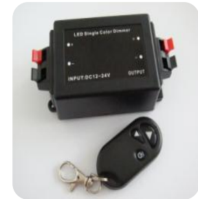
RF Strip Controller
