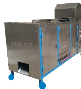
SEMI AUTOMATIC CHAPATI MAKING MACHINE Production capacity (per hour) - 500-750-1000
