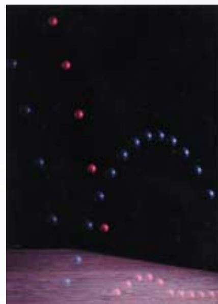
Red: HYBRAR™ based compound Blue: Common rubber based compound
