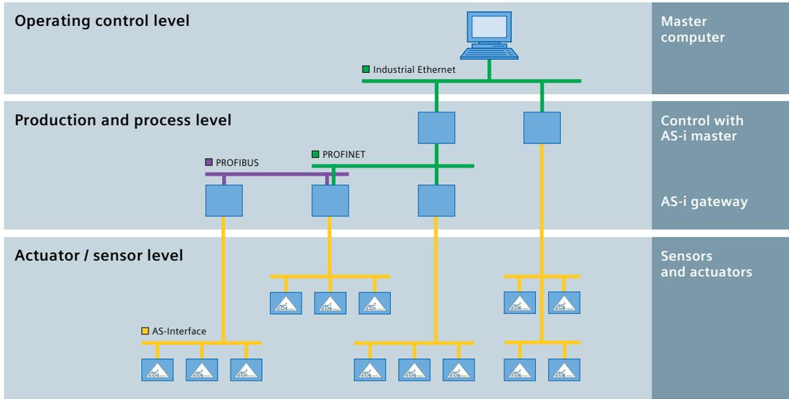
The assembly of a complex automation system is not easily comprehensible at first sight. Particularly the field level, which features a large number of realtime-capable devices, requires a clear structure.
