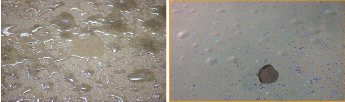
**Conventional epoxy coating on green (Fresh) concrete is failed due to De bonding, blistering and delamination**
