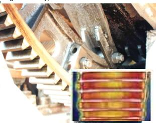
evaluation of reducer, main motor and couplings state; thermal image analysis in that case is focused on the areas of: bearings, shaft seals and couplings; all areas of significantly increased temperature may point on the abnormalities like for example: bearing's failure and/or improper lubrication, improper functioning of the sealing and/or its improper lubrication, damages of coupling elements and/or improper exploitation conditions (like incorrect shafts alignment).
