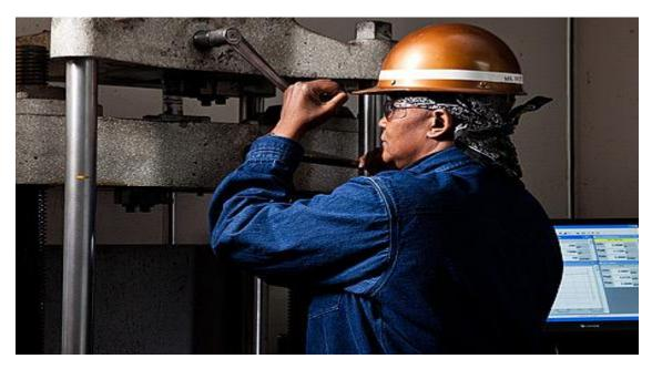
ITE is accredited by NABL in the field of Mechanical & Chemical Testing of Metals. This division is responsible for looking after activities like tensile tests, bend tests, spectro/chemical analysis, hardness test, impact test, welder qualification and other destructive testing services.
