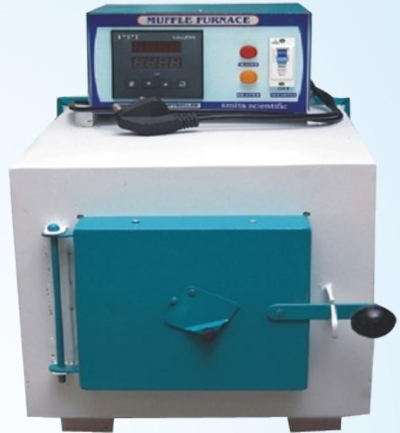
**HEATING ELEMENTS AND TEMPERATURE CONTROLLER:** Silicon carbide heating elements are fitted to achieve the temperature upto 1400°C. The temperature is controlled by FUJI/ HONEYWELL / MEXTHERM PID Microprocessor based Digital Temperature Indicator cum controller with temperature stability of  $\pm 1^\circ\text{C}$ . The controller with 8 programmes and 4 step in each segment with ramp and soak to display the set temperature with dwell auto cut off at set point.
