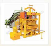
Stationary Block Making machine is hydralic operated, semi Automatic with hooper, Mix Reeder, Pallet Pusher.
