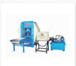
A Fully automatic fly ash brick making machine with 150 ton pressing capacity this machine eliminates the need of wooden pallets. The bricks can be removed at the same time of manufacturing. This machine is controlled by PLC.
