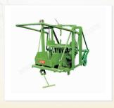
This is an egg-laying type manually Operated Concrete Block Making Machine on wheels, which after laying a block on the concrete floor is moved to the next laying by manual force. Different type of concrete blocks can be produced with consistent quality by fixing different types of concrete mould and ram into the machine.
