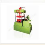
This machine is used to make high density paving blocks. This machine eliminates the need of wooden pallets. The adjustable Height is 2" to 4".
