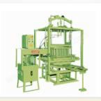
This is a stand type Hydraulic operated Concrete Block Making Machine with a high Frequency Vibrator. The block is made with the help of Wooden / Steel Pallet. Any type of concrete block can be produced with consistent quality by fixing required type of concrete mould and ram into the machine.
