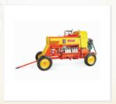
This compact machine is a mobile clay bric-making machine. With th help of SS moulds really good quality bricks can be made. The clay when poured into the drum, the material will be crushed and moulded. Both clay crushing and mould washing is done by one drive.
