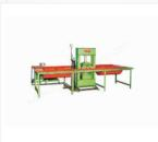
This is a versatile machine which is used to make Mosaic Tiles and Paving Blocks. This machine also eliminates the need of the wooden pallet.
