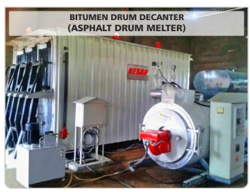
KESAR decanters are designed for ease of operation & provide the most efficient system for ensuring a high throughput of drummed bitumen. Designed for use in association with bulk storage tanks the melted bitumen is automatically transferred from the decanter reservoir to the storage tank during the decanting process.
