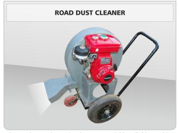
The Road Dust Cleaner is a low cost & Highly Reliable Machine. The Machine Build Specifically for road dust cleaning for WBM, WMM & Asphalted Road Surface Applications with simple operating system. (As per Specification of MORTH)
