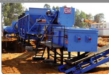
KESAR Wet Mix Plant is Suitable for Wet Mix Macadam & sub base. The Plant Provides higher production in low cost with Automatic control of Wet Mix Material as per the latest MORTH (Ministry of Road Transport & Highway) specification. The Standard configuration of the plants comprise of the following units:
