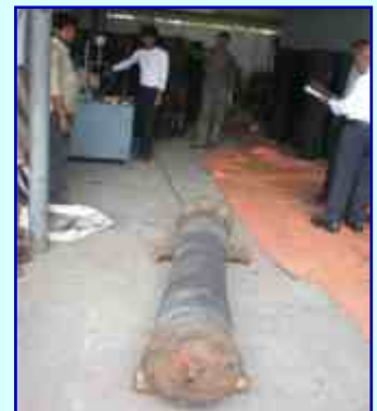
DREDGE HOSE UNDER HYDROSTATIC TESTING
