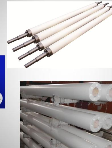
Fused silica hollow rollers are used in silicon steel annealing furnaces as bottom rollers, replacing traditional graphite carbon housing and ceramic coating rollers to solve the problems of surface oxidation, nodulation, etc. It can avoid frequent replacement of rollers, promoting production efficiency and steel sheet surface quality.
