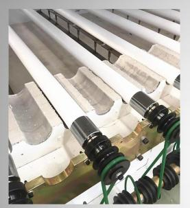
Fused silica rolls for horizontal glass tempering furnaces are key components of glass horizontal tempering furnaces for glass support and transportation. It's better to increase the productivity and quality in good condition of installation, using and maintenance. Premium quality tempered glass requires premium quality rollers. We can supply good quantity fused silica roller according to customers' furnaces requirements.
