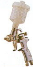
SG - 08 (Cup Capacity : 0.125ltr) High Volume Low Pressure Gravity Feed Spray Gun Air Pressure : 40-45 psi, Weight : 0.5 kg Optional Nozzle : 0.5,0.8,1.1,2.0 mm
