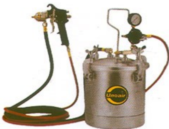
SG - 80 (Cup Capacity : 10 ltr) Heavy Duty Industrial Paint Spray Gun (Pressure type) Air Pressure : 30-80 psi, Weight : 11 kg Standard Nozzle : 1 mm
