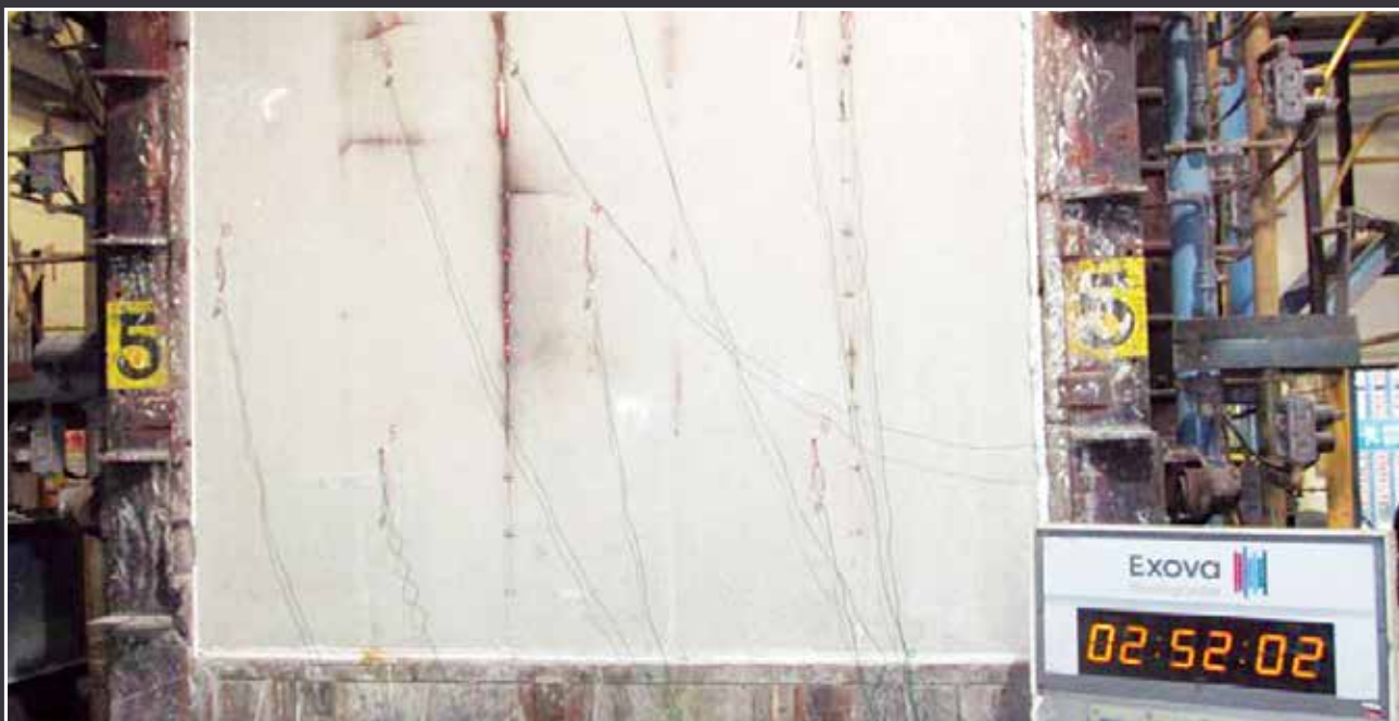
Exova Warrington fire rating test
